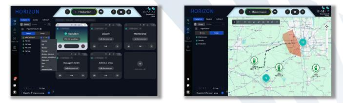
Dispatch applications can track multiple user locations and travel routes with job site time stamps to manage and dispatch vehicle fleets and remote workers. Dispatchers can draw geofences on the map to define boundaries for territories and service areas. Alarms can be generated when users enter or leave geofenced areas.
